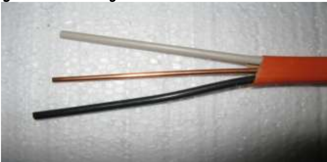
This is 10-2 with ground, 1 hot, neutral and bare ground. Orange jacket.
