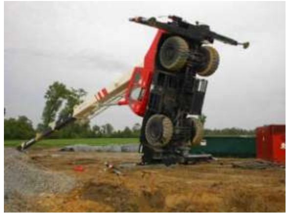
This is the results of over extension. Think of you in that cab, I've been there.
